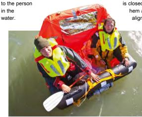
Four large, weighted ballast bags hold it steady in the water and she is easy enough to right when upside down using the grab line provided. Boarding was not particularly easy thanks to the lack of a long ladder or line inside. So, though it does have weighted webbing steps on the outside and a single grab strop on the inside of the tube at the front, you have to stretch for the webbing lines around the inside of the tubes to pull yourself in. Once inside the large canopy
